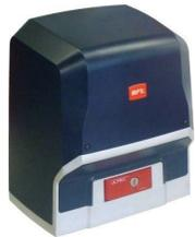
This 24V motor operates sliding gates up to 1000kg or 1500kg in weight and with a leaf speed of 9m/min or 12m/min (Fast version). Magnetic limit switches, personalised key for manual release and U-Link control board with display. Approximately 150 operations a day. U-LINK READY.
